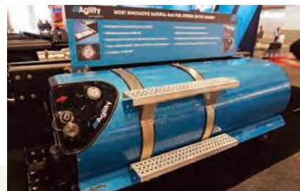
An Agility Fuel Systems LNG fuel tank at an industry trade show
