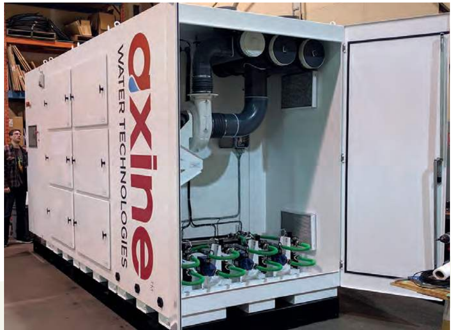
Axine modular water treatment systems are wirelessly connected and remotely monitored
